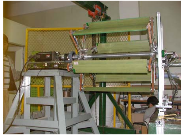
Fig. 21 Test model of cycloidal blades system
