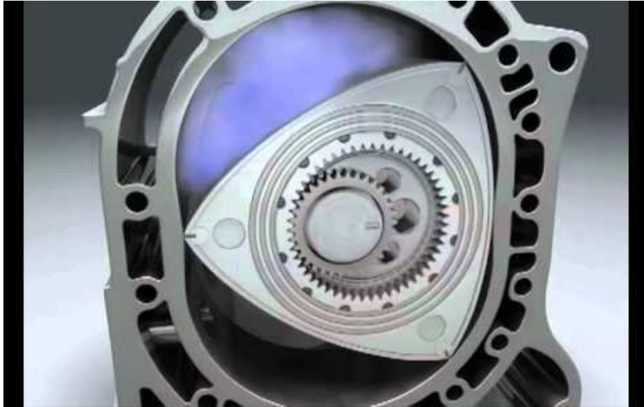
Fig. 1. Wankel engine with open lid, somewhat obliquely photographed. Please note the contact of the seal with the inner surface of the chamber on the left. If the curvature of the side wall is positive at the contact point, then the curvature at the contact points of two other sealing elements is negative. In the places where the positive curvature changes to the negative, the centrifugal force abruptly tips over, and the sealing lip chops into the inside of the chamber like an axe. See fragment e ) in the explanation below.
