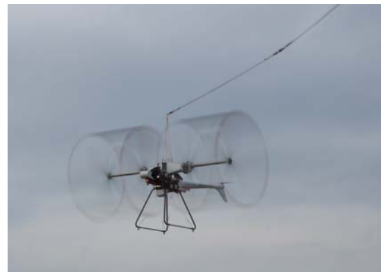
Fig. 11 Stable hover flight of the cyclocopter
