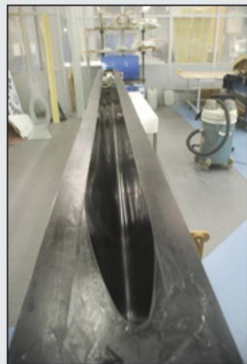
**Bonding the "leading-edge" ribs to the main spar.**
