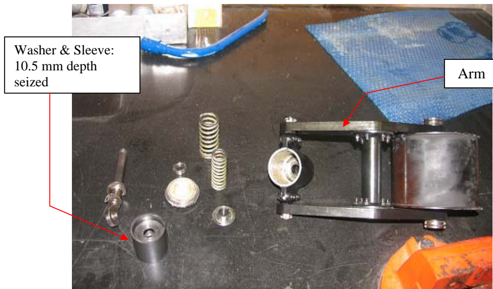
Photo 3 shows the disassembled Idler Actuator
