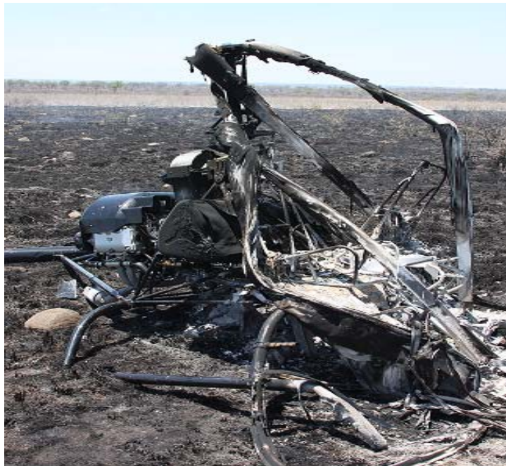
Photo1: Shows the fire damage caused to the helicopter.
