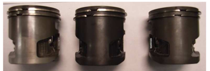
Figure 10. Intake side of the standard piston (left) after engine test 1, the DLC-1 coated piston (middle) after engine test 4 and the W-DLC coated piston (right) after engine test 5.
