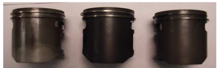
Figure 9. Exhaust side of the standard piston (left) after engine test 1, the DLC-1 coated piston (middle) after engine test 4 and the W-DLC coated piston (right) after engine test 5.
