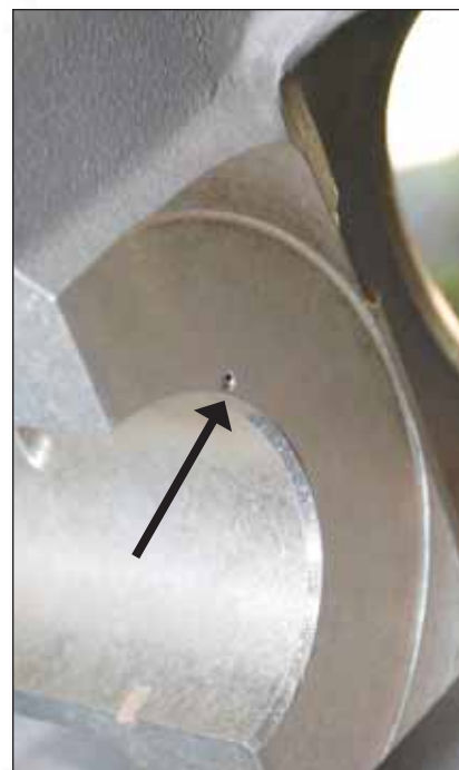
Superior's XP-360 engine uses pressurized thrust-face lubrication. Oil is delivered to the face through the small passage indicated by the arrow. This technique ensures that the face of the crankshaft will have sufficient lubrication.
