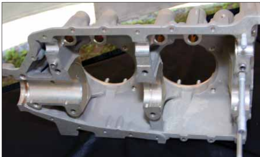
A case in point: Superior's cases are designed to be compatible with basic Lycoming components but offer several improvements. For example, the webbing between the adjacent cylinders is thicker than on a standard Lycoming part. Mounting bosses for oil-squirt jets aimed at the pistons are standard.
