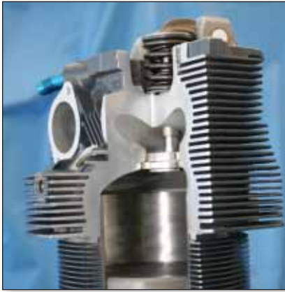
ECI's Titan cylinder assemblies incorporate strengthening and durability strategies, including high-chrome valve guides.
