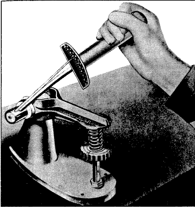
Fig. 83—Checking Valve Spring Tension
