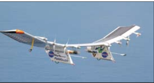
Paul MacCready's Pathfinder ran its eight electric motors from lithium ion batteries recharged by solar cells atop the wing.
