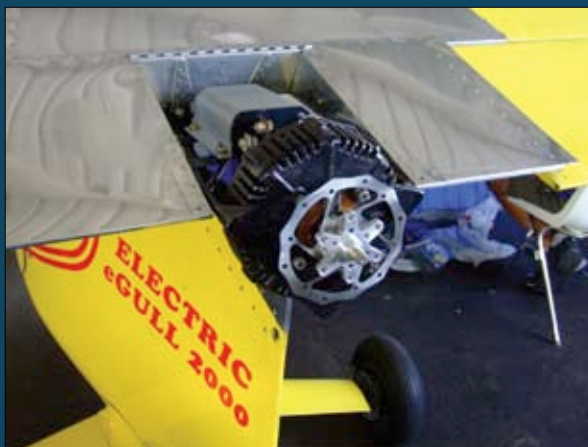
Mark Beierle's eGull 2000, when equipped with its PowerFin propeller, has lofted him more than an hour on a battery charge.
