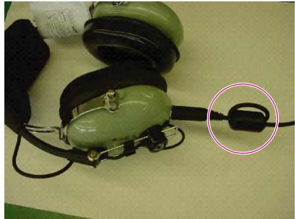
Note: Cross the wire inside the core when installing.
