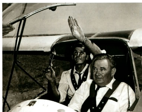
This photograph shows the staggered seating arrangement with the instructor behind and to one side of the pupil.
