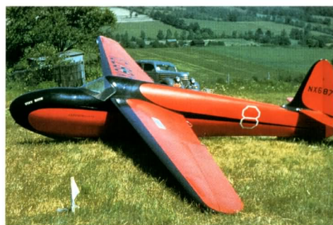
Above, the Tiny Mite before and, right, after the transformation. The best glide ratio was increased from less than 20:1 to more than 30.
