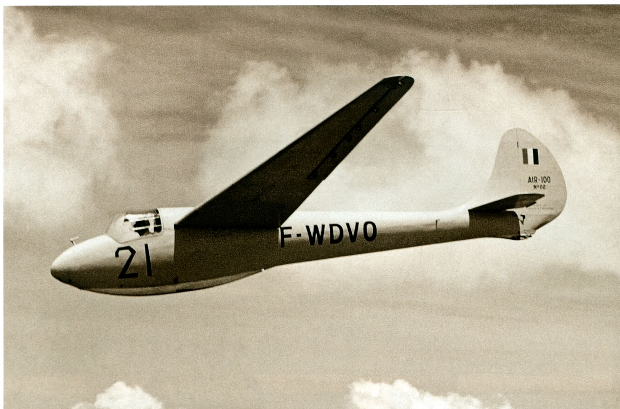
Left: The Arsenal Air 100 of 1947 was similar in general design and appearance to the German Weihe of 1938, but it had many detailed improvements and was slightly heavier.
