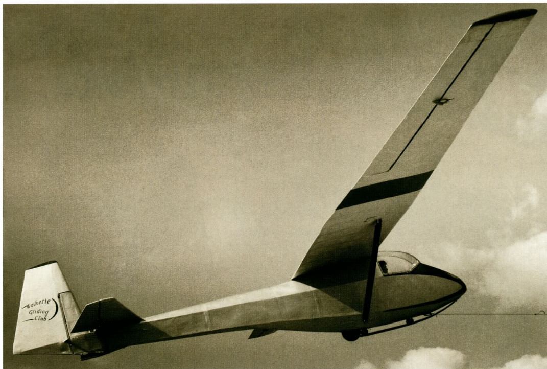
Above: The later Grunau Baby 4 had a blown plastic canopy and rounded front decking. This example was restored and flown in 1997.
