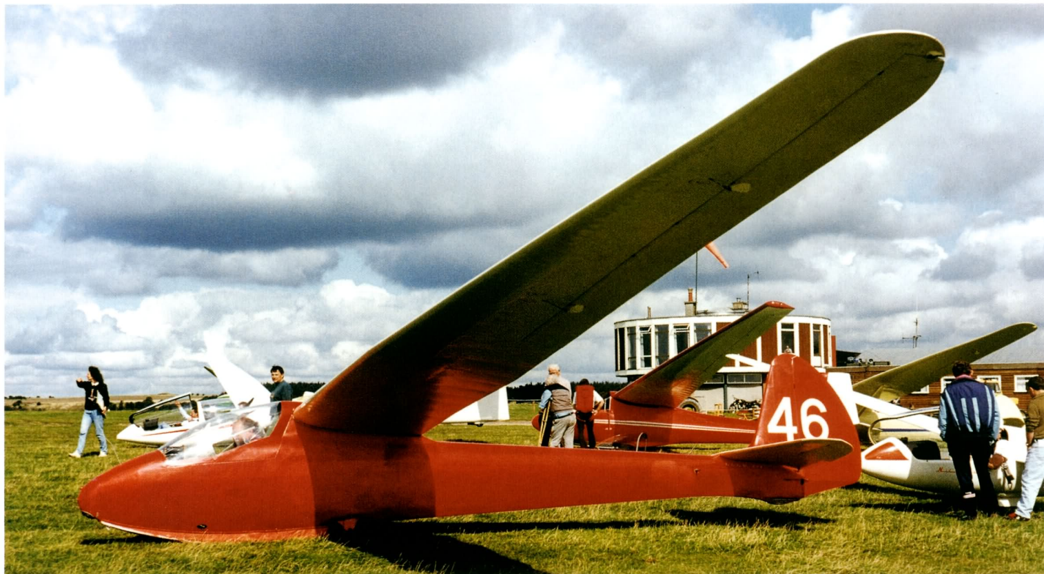
Above: Slingsby's answer to the Weihe was an eighteen metre span version of the T 25 Gull IV. The T - 34 'Sky' flew first in 1950. This one is at Sutton Bank in Yorkshire Left: The name 'Sky', is said to have come from the initial letters, Slingsby, Kirbymoorside, Yorkshire. Several of the type survive and are capable of excellent flights
