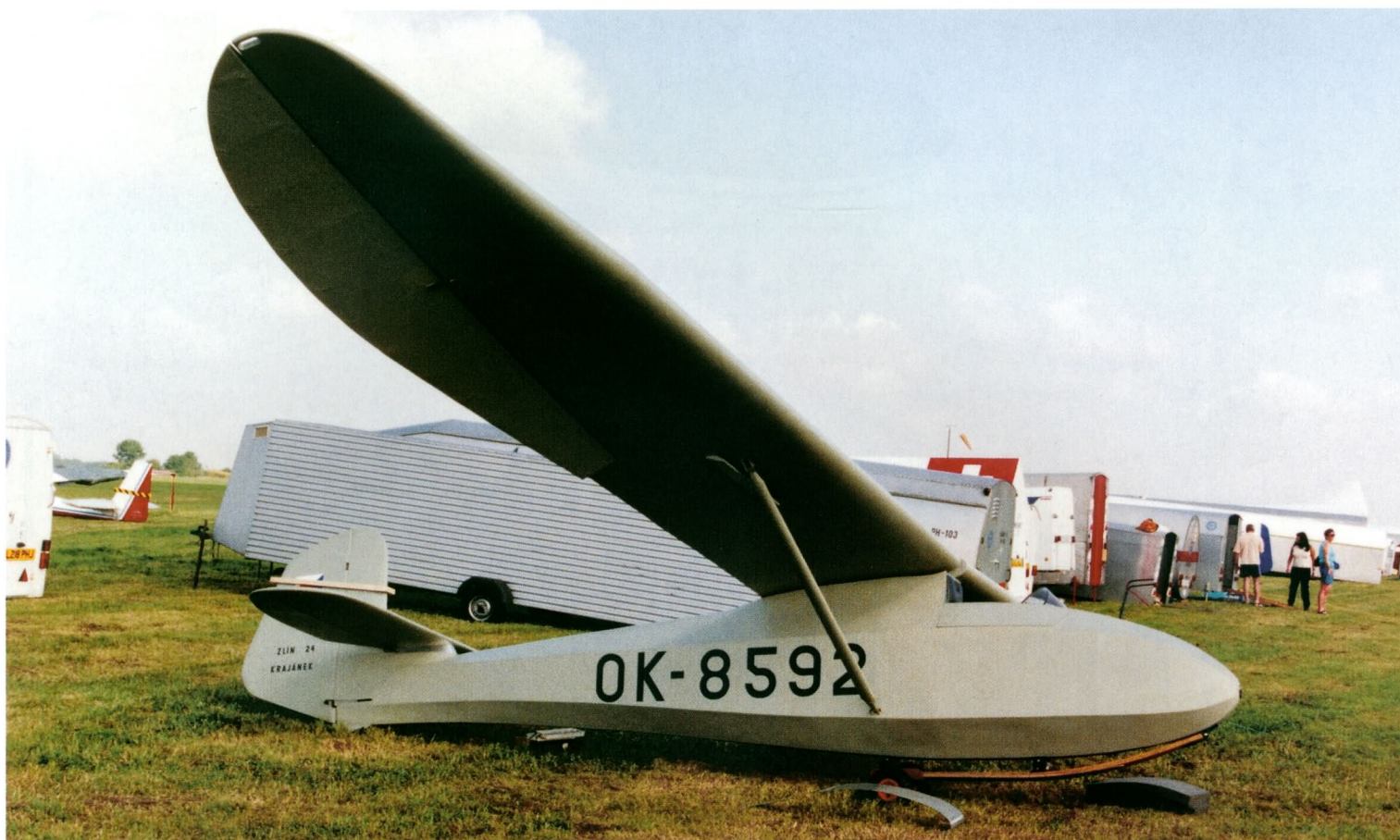
In appearance not unlike a Grunau Baby, the Zlin - 24 Krajanek was stronger and stressed for inverted flight. The surviving Krajanek has made regular appearances at vintage rallies in recent times.
