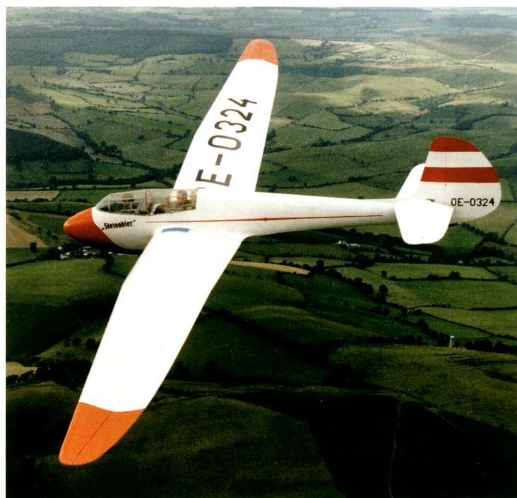
The Mg 19a, with gull wings, has slightly improved ground clearance.
