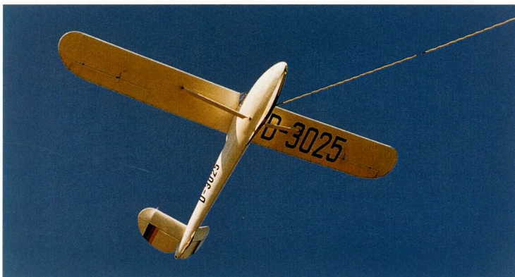
Above: The Ka - 3 was similar to the Ka - 1 but had a welded steel tube fuselage frame, marketed as a unit with the kit.
