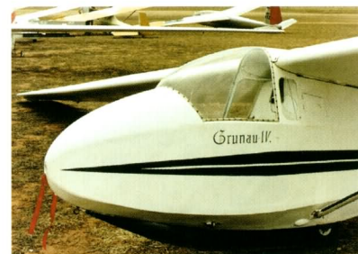
Above: The later Grunau Baby 4 had a blown plastic canopy and rounded front decking. This example was restored and flown in 1997.
