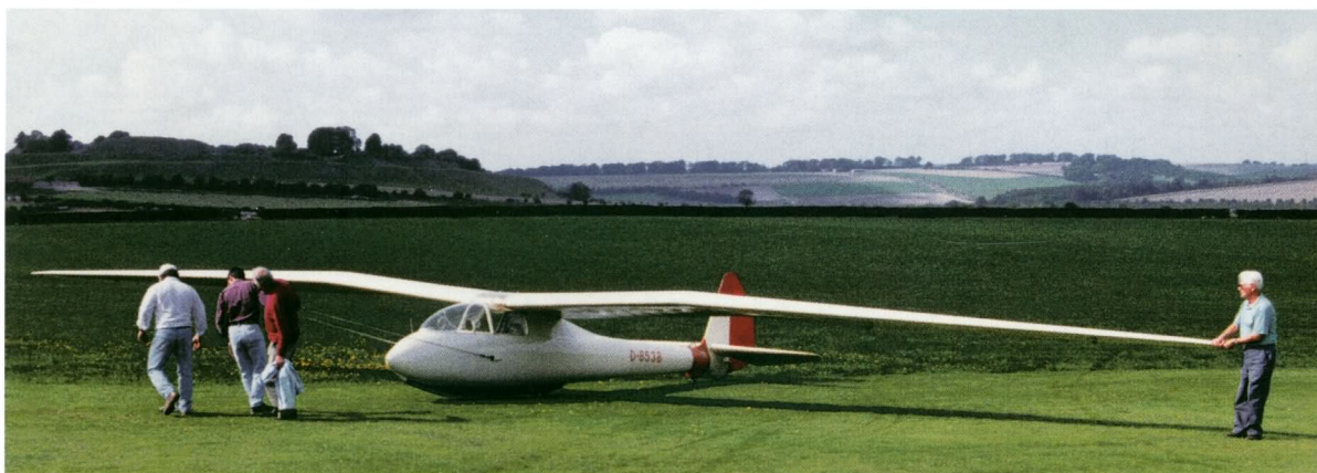
The Condor IV, as it first appeared with a narrow fuselage neck to support the wing. Several of the type were flown at Madrid in 1952.
