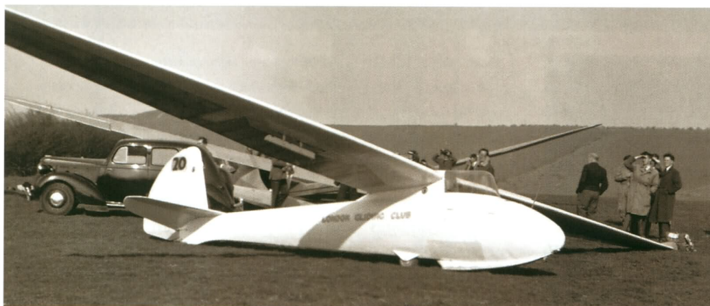
Above: The only surviving Gull IV has a Kite 2 fuselage adapted.
