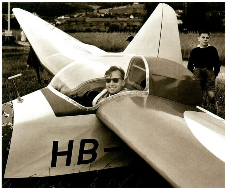
Later versions of the AV - 36 had improved cockpit canopies. This is number 111.
