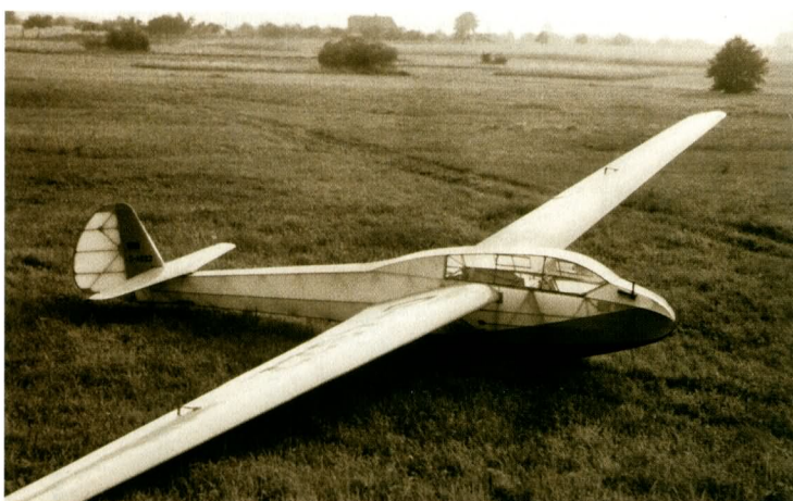
Above: The rounded fin and rudder show the earliest form of the Mu 13E. The photo was taken at Porta Westfalica near Minden.
