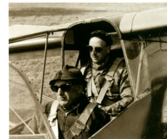
The Polyt III two seater was designed and built by students of the Polytechnic flying club in Denmark. The instructor's seat was raised to improve the forward view. Later modifications included a shortened fuselage
