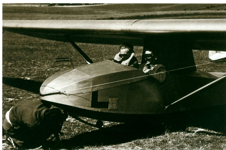
Above: The Type 21 prototype in 1944 as it was originally intended to be. For early flights it was thought the pupil must feel the airflow, as with a primary glider.
