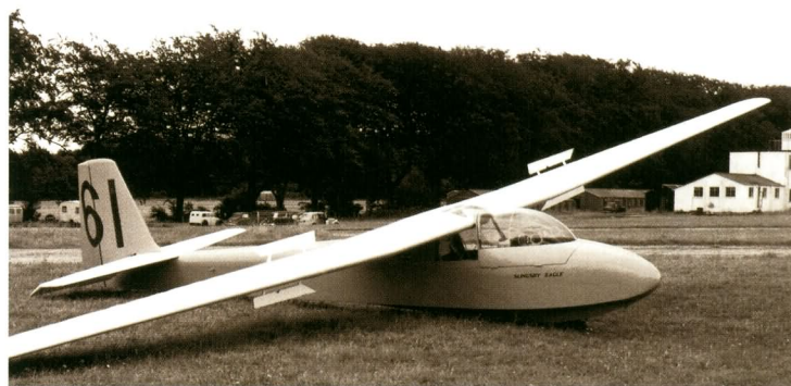
Improvements and simplification of the design, led to the Eagle 3, which had a straight leading edge and the airbrakes moved to the outer section of the three-piece wing.
