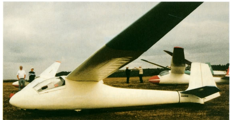
Top: The Skylark 2 was a complete redesign of the Skylark 1 with new wing of greater span and an improved fuselage. More of the Skylark 2 were built than any previous Slingsby high performance sailplane. Many had canopies altered in service Above: Skylark 2 with a Skylark 3 behind.
