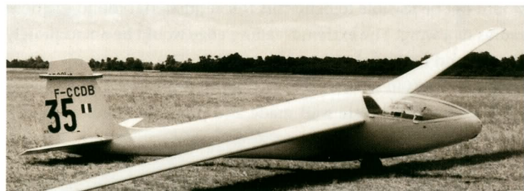
Top: The graceful fuselage lines and the elaborate external flap hinges of the early versions of the Breguet 901, are displayed here. This was an early production aircraft.
