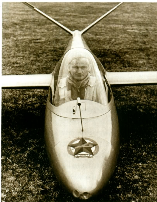
An unusual picture of the pilot in the cockpit of the OMRE OE - 1. For 18 metres span the wing was extremely thin. As the drawing shows, an exceptionally strong main spar was needed
