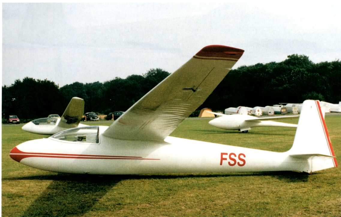
The Ka 6E, with refined fuselage and cockpit and an all-moving tailplane, was the final version of the Ka 6. This was at Lasham in 1992.
