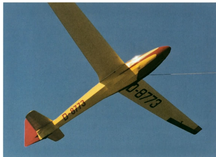
Below: The Zugvogel 1 has swept forward wings, distinguishing it from the later Zugvogels 2, 3 & 4.
