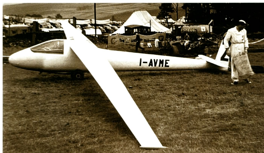
Right: The Spillo at Camphill in 1954. The wheeled dolly was used for take off but on the rough Derbyshire fields the small skid undercarriage proved inadequate for landings.
