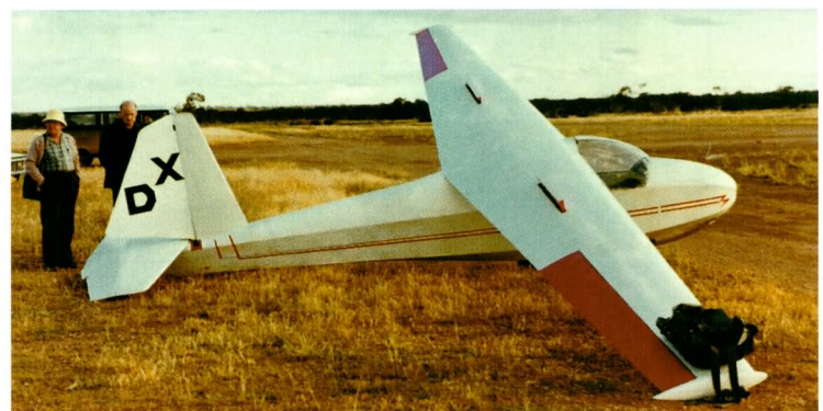
Above: The ES 54 Gnome was an experiment with a very small, light sailplane. It flew successfully in June 1955 but performance was very limited and no orders were received. Right: The ES 56 Nymph with a NACA six digit wing profile, performed well for its size and pilots liked it, but only four were built
