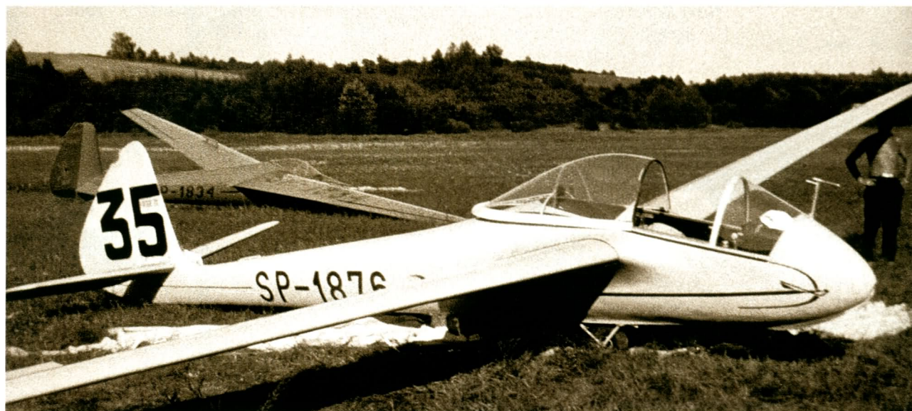
The later versions of the Jaskolka, SZD - 8 - ter ZO, had a smooth shape for the nose and front cockpit canopy. The canopy slid back on rails to allow access to the cockpit.
