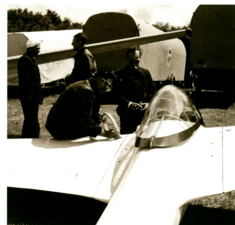
Above: The Jaskolka - 8 - bis W was fitted with water ballast tanks, here being filled before a contest flight. Left: The V tailed SZD - 17X Jaskolka L in the museum at Krakow. Photo V Pedrielli
