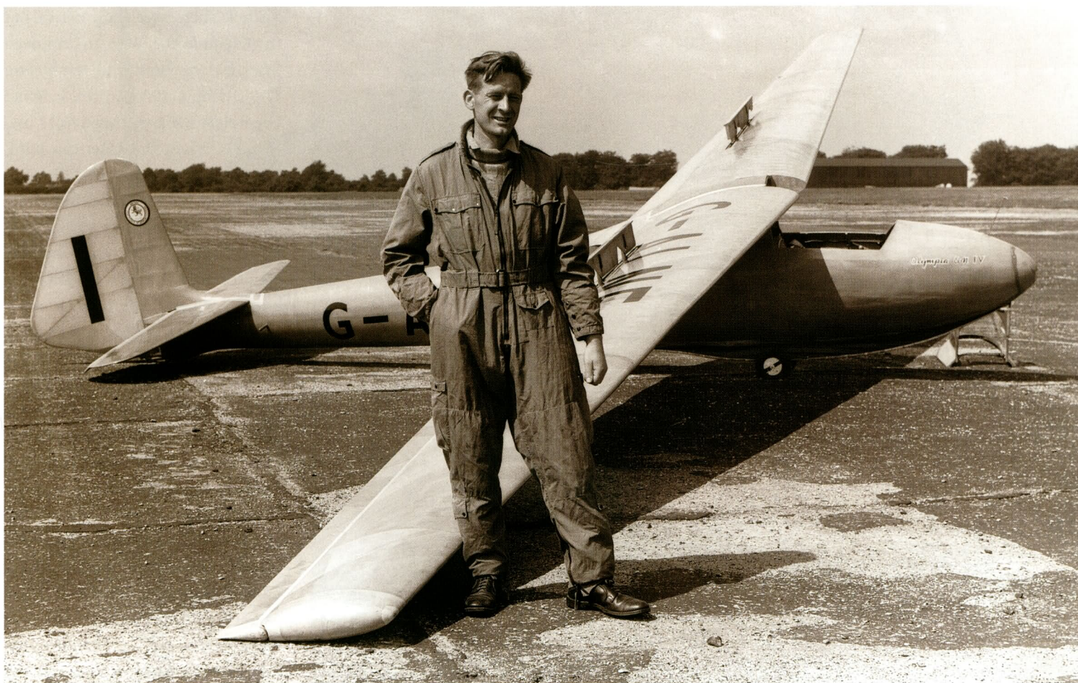
Top and right: The Olympia 4 had a new 'laminar' wing with NACA 64 3 618 profile. The fuselage and tail were adapted from an ordinary Olympia. Geoffrey Stephenson at the 1954 World Championships at Camphill flew it in this form. The photograph above shows David Ince, the test pilot for Elliotts.
