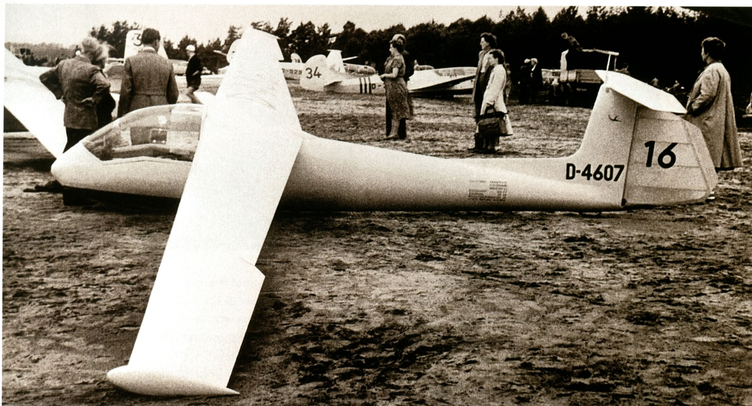
Top: The Darmstadt D - 34a, with T tail, first of a series of small experimental sailplanes. Ailerons, tail and cockpit were all considerably modified in service.
