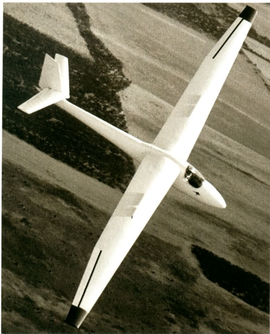
Above: The Super Arrow, ES 60B, a slightly downgraded version of the ES 60 Left: The ES 60 'Boomerang' was very successful in Australian conditions and set many national records. It was entered for the OSTIV Standard Class design contest in 1965 but was ruled out by a fractional error in the wing span.
