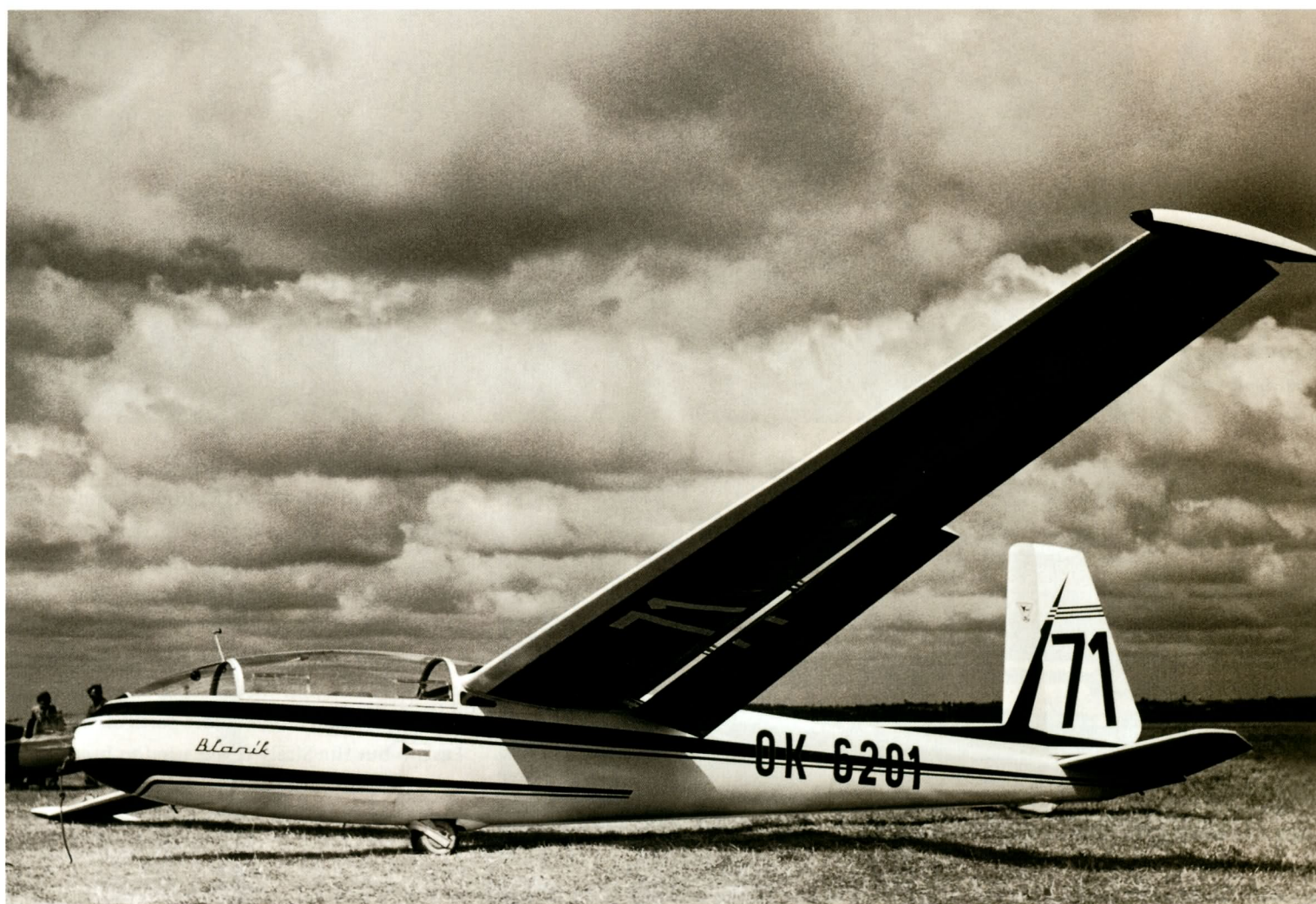
Above: The Blanik had large Fowler type flaps, shown here extended. Note also the shoulder type tow releases on this early production example
