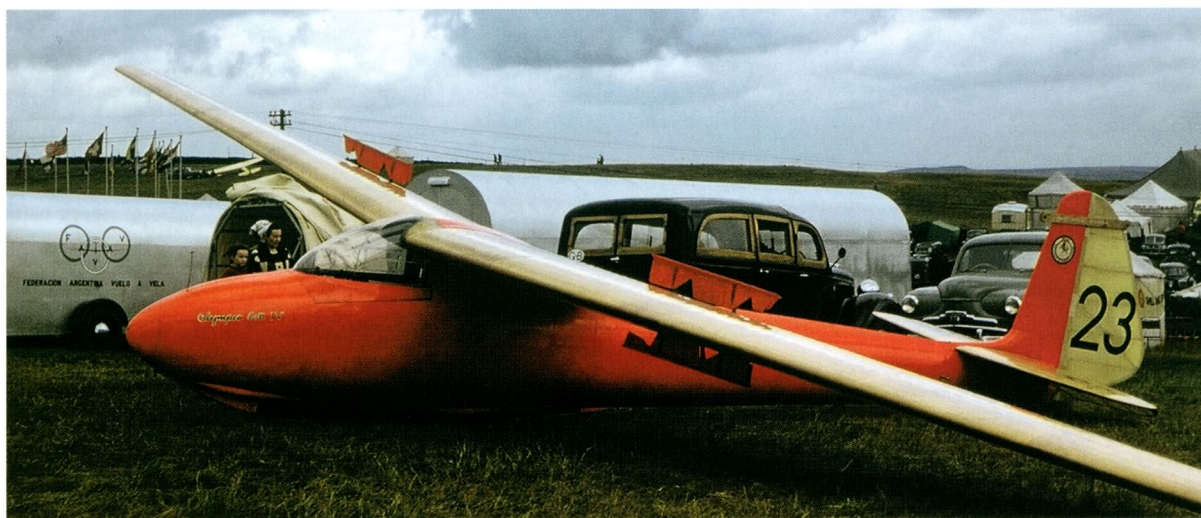
Top and right: The Olympia 4 had a new 'laminar' wing with NACA 64 3 618 profile. The fuselage and tail were adapted from an ordinary Olympia. Geoffrey Stephenson at the 1954 World Championships at Camphill flew it in this form. The photograph above shows David Ince, the test pilot for Elliotts.
