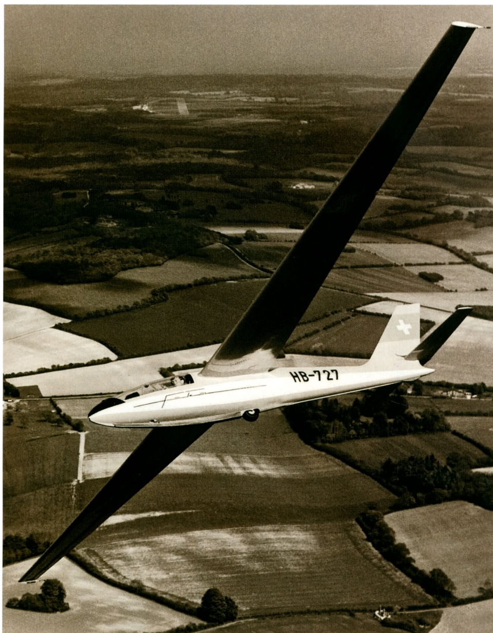
A Swiss registered Foka 4 flying over England. The wheel, set far into the belly, made ground handling rather difficult. This counted against it in the OSTIV Design Prize judgment
