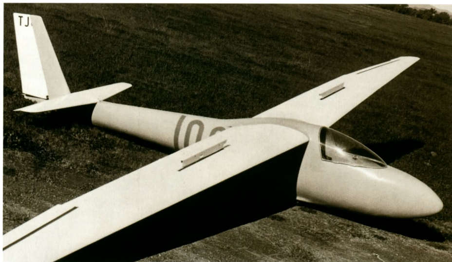
Above: The Super Arrow, ES 60B, a slightly downgraded version of the ES 60 Left: The ES 60 'Boomerang' was very successful in Australian conditions and set many national records. It was entered for the OSTIV Standard Class design contest in 1965 but was ruled out by a fractional error in the wing span.
