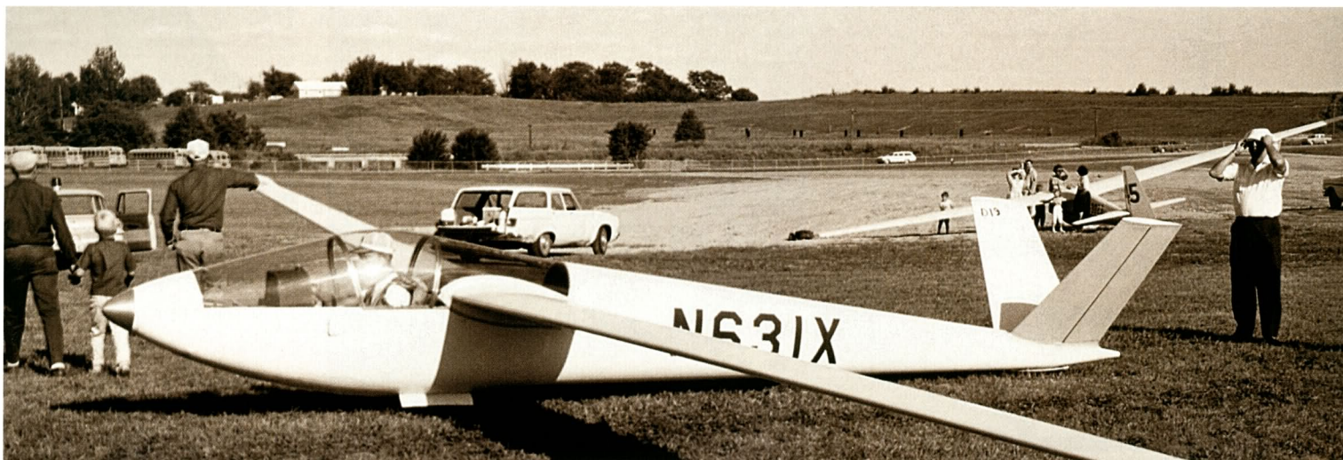
Above: The HP - 11a, with retracting wheel, seen in 1964
