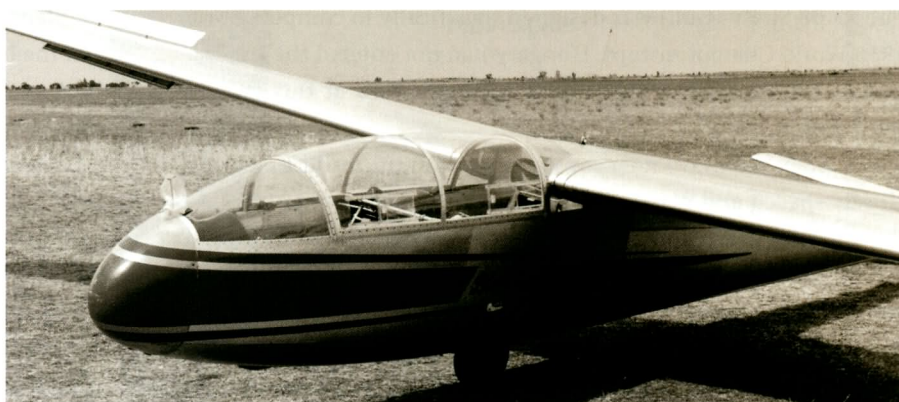
Above: The Blanik had large Fowler type flaps, shown here extended. Note also the shoulder type tow releases on this early production example
