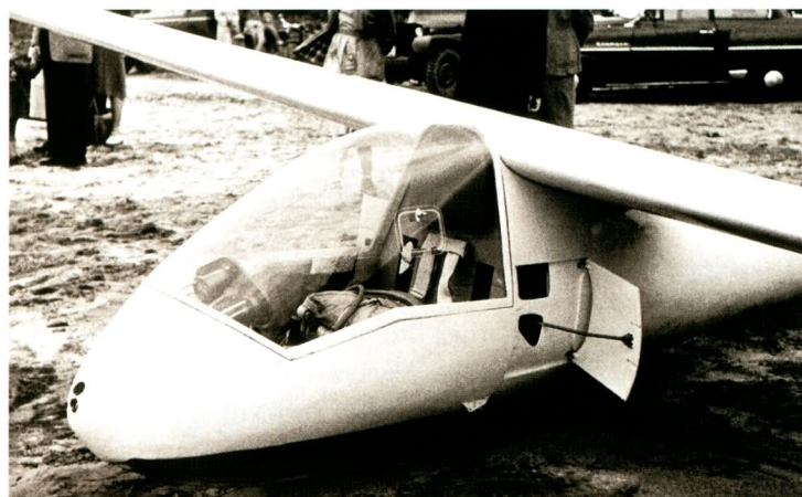
The air brakes of the D - 34 were in the fuselage behind the cockpit
