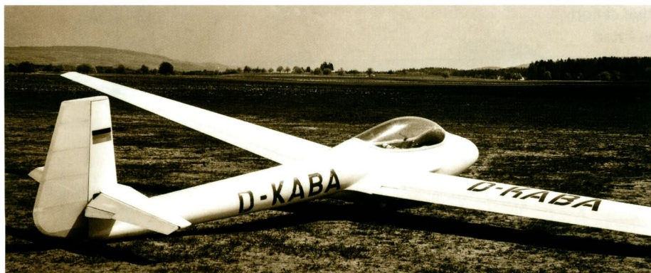
The Hütter 30 - TS, turbine powered originally but soon converted to a sailplane
