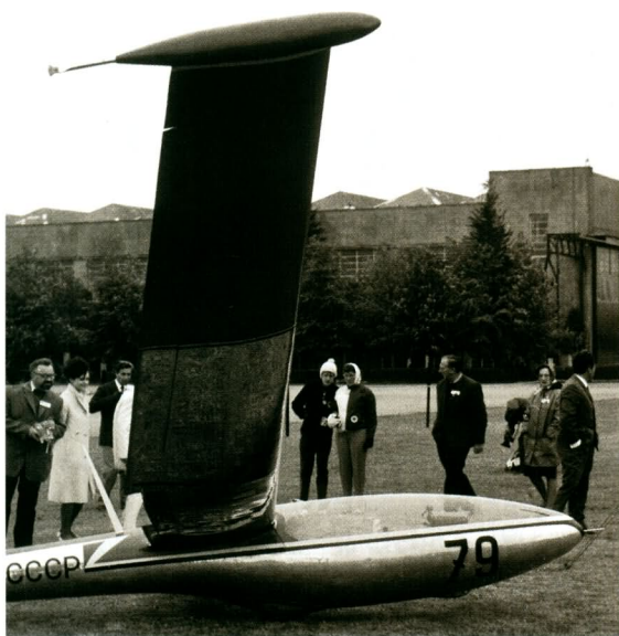
The extraordinary KAI 14 entered by the USSR at South Cerney. The poor forward view from the cockpit contributed to accidents
