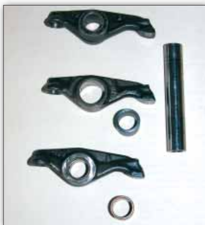
From top to bottom (as oldest to newest) are the various rocker-arm configurations used by Rotax. The top has the original steel bushing at the pivot. In the middle is the phenolic version that replaced the steel; it is still considered a serviceable part. At the bottom is the latest bronze bushing. The rocker shaft (at right) shows minor wear patterns.
