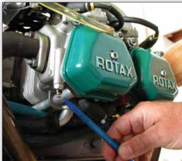
This is one of the two CHT probe locations on the 912. If the thermocouple is melted, the engine has seen a severe overheating and requires a thorough examination before being put into service.
